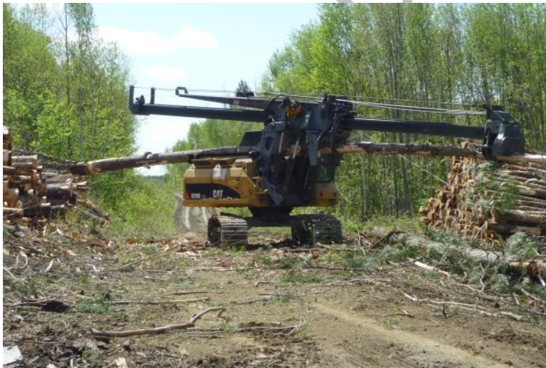
101 102 Figure 1: A stroke delimiter generally processes one tree at a time by cutting of branches and the top 103 above a specific merchantable diameter.
