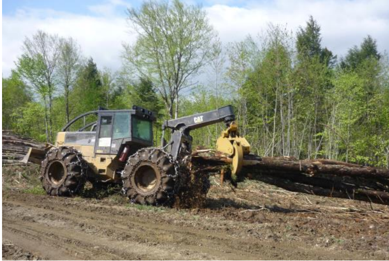
105 106 Figure 2: A grapple skidder generally transports several trees in a bunch from the forest to the roadside 107 where the whole trees get processed by a stroke delimeter.
